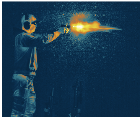
Figure 3: The thermal infrared signature (3.0-5.0 \mu\text{m} ) of a 9mm pistol muzzle flash as captured by the M700 HDR camera. All-new on chip saturation management functionality allows for a snapshot dynamic range of more than 900C to be captured in a single image with a single optical path and exposure time. This provides superior data quality without concerns owed to low signal or saturation.
